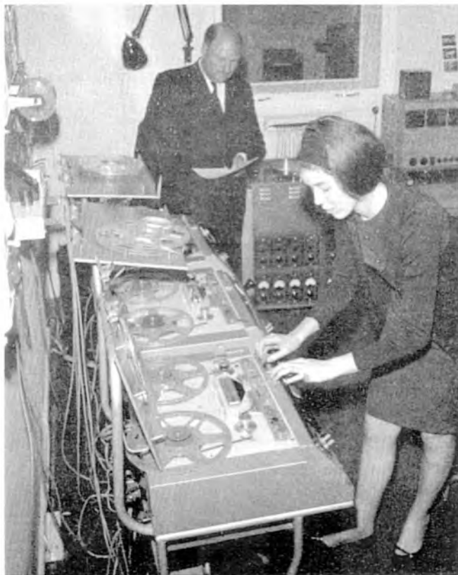
Using a simple editing block and razor blade, Delia Derbyshire edits a musical note on tape while Desmond Briscoe consults the score. A typical working area at the Radiophonic Workshop
